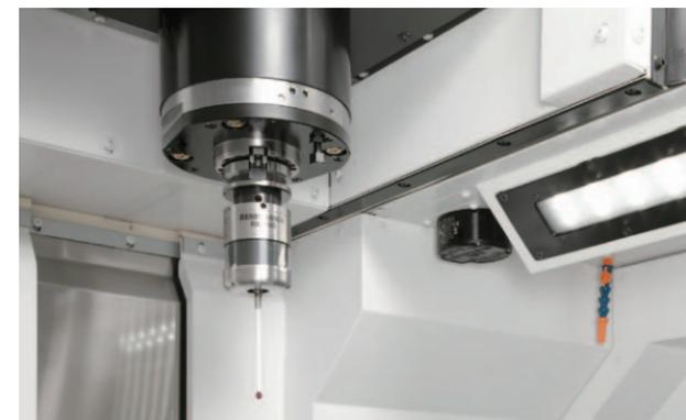
●刀具折损检测、自动刀具长度补偿
